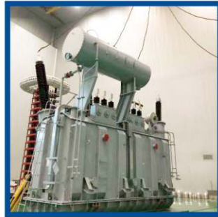
900MVA & 60MVA, 220kV power transformer for 900MW liquified natural gas power projects of Ministry of Electricity and Energy of the Government of Myanmar
