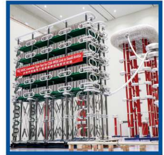
2 sets ±500kV/3000MW VSC-HVDC converter valves for Riyadh-Jeddah HVDC project, Saudi Arabia
